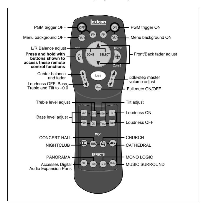
MC-1 Digital Controller Installation
